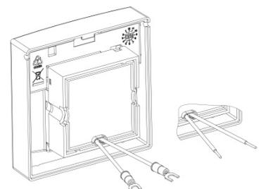
The MCP is installed by locating the upper mounting hook into the receiver in the back box and then pushing the unit gently home. The single fixing screw may then be tightened as required.
