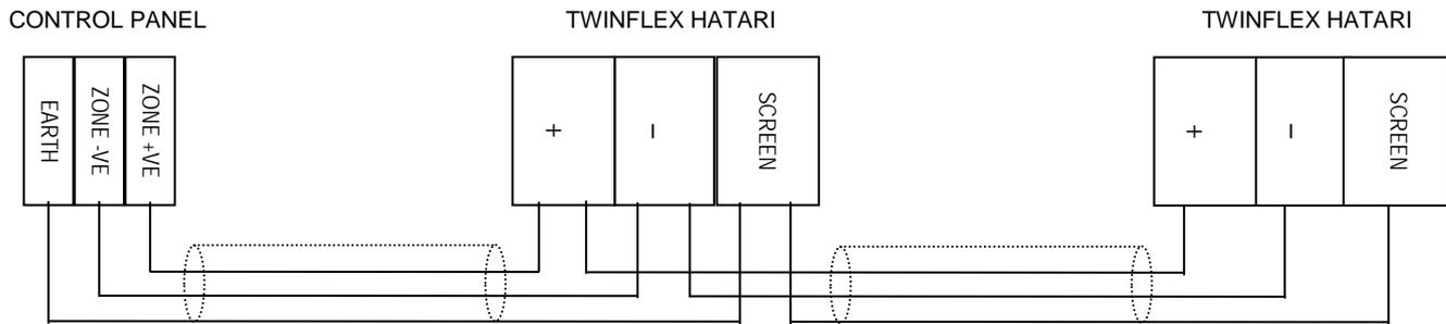
The Twinflex Hatari Sounder can be mixed on the same zone as other types of Twinflex device (eg. Twinflex Multipoint Detectors). The above diagram shows how to make the zone positive, zone negative and screen connections between the control panel and Twinflex Hatari Sounders. Refer to the instruction leaflets supplied with other Twinflex devices for their equivalent wiring/terminal labelling details.
